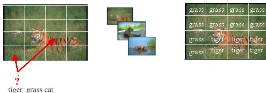
Figure 3: The correspondence problem between image regions and words: The words tiger and grass are associated with the image, but the word-to-region correspondences are unknown. If there are other images, the correct correspondences can be learned and used to automatically label each region in the image with correct words or to auto-annotate a given image.
