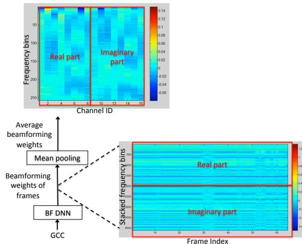
they are optimal in predicting the clean magnitude spectrum, which is closer to the speech recognition task. In the third step, the acoustic model network is trained using the beamformed features. In the last step, the two networks are jointly trained with a large learning rate such that the networks can jump out of local minima caused by the previous steps and find a better set of weights.
